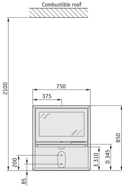
The minimum distance in front of the stove opening to combustible parts of the building or interior decoration must be at least 1,4 m.
