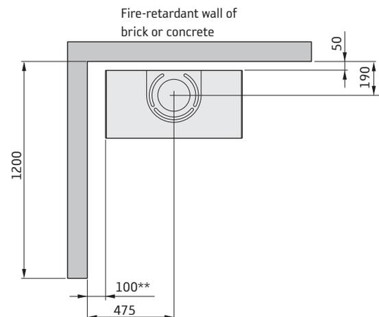
\* If the stove is placed on a hearth plate made of glass for example (accessory), the height from the floor is affected by a distance corresponding to the thickness of the hearth plate, for a free standing glass hearth plate this is 10 mm.
